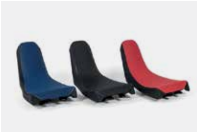
LOW SEATS 08R73-MKS-E00ZA / 08R73-MKS-E00ZB / 08R73-MKS-E00ZC The Low Seats reduce the seat height by 25mm. Depending on the position selected, the result is a seat height of 825 or 845mm. Available versions: • 08R73-MKS-E00ZA: Red version • 08R73-MKS-E00ZB: Tricolour version • 08R73-MKS-E00ZC: Black version
