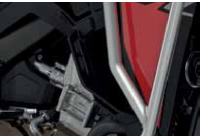
DEFLECTORS SET 08R72-MKS-E00 The deflectors improve comfort by reducing travelling air around the rider's waist and knees while funnelling the warm air emitted by the radiators.
