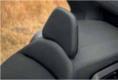
RIDER BACKREST 08R75-MKC-A01 High-quality backrest with embossed Gold Wing logo. It provides extra comfort to the rider and tilts forward to ease the passenger access. Not compatible with Custom Seat.
