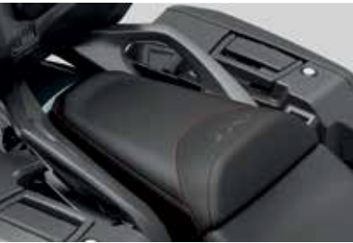
COMFORT PILLION SEAT 08R73-MLF-E00ZA Thanks to its softer construction and its increased 15mm thickness, this pillion seat provides an extra level of comfort enhancing the riding experience.
