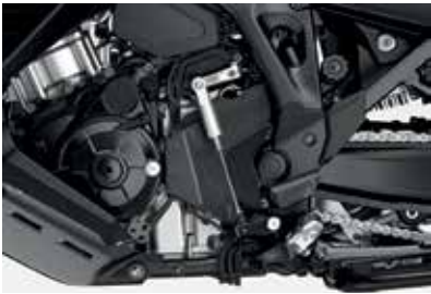
QUICK SHIFTER 08U70-MLF-E00 Only applicable to manual transmission versions of the NT1100, the quick shifter enables smooth but instantaneous clutchless gear shifts, both up and down. For an increased comfort and added sportiness of the riding experience.
